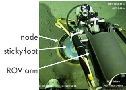
Figure 1: Node depth measurement on an OBN using a sticky foot on an ROV arm
