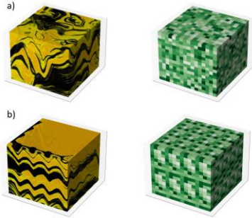
Figure 4: a) A random 128 \text{ m} \times 3200 \text{ m} \times 3200 \text{ m} sample from a trained GAN (left) together with the corresponding latent space coordinate (right), padding voxels omitted for clarity. b) A GAN sample generated from a latent coordinate manually constructed by tiling the smaller latent coordinates from Fig. 3b-c.
