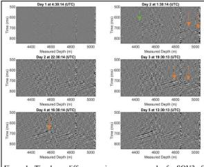
Figure 1: Timelapse difference seismogram examples for SOV3 of continuous operation as acquired in the monitor well. Day one is before treatment and the seismogram shows residual noise. A series of scattering events appear from the direct P as treatment commences in the injection well (Correa et al., 2024).
